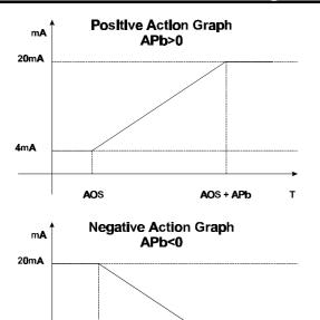
NOTE: When the defrost is in progress, the analogue output is set to the minimum value (4 mA). This condition lasts until the defrost terminates
